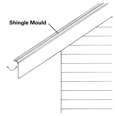
Sloped Boxed Eave Rake Detail
